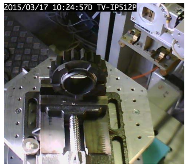
Fig. 4. Photography of the welded gear. Right: photo made during the experiment
