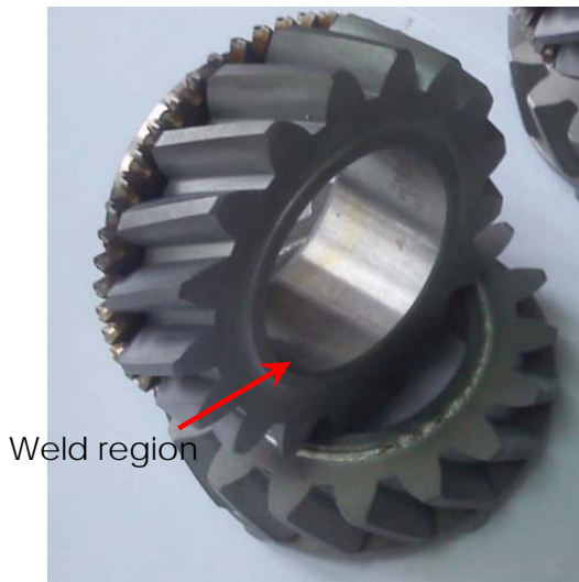
Fig. 4. Photography of the welded gear. Right: photo made during the experiment
